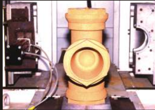
Laempe Core shooters with 5 ,10 , 40 Litre capacity
