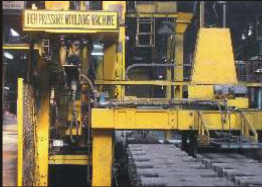
Flaskless High pressure Moulding Line (820x820x560mm @ 90 moulds/hr)
