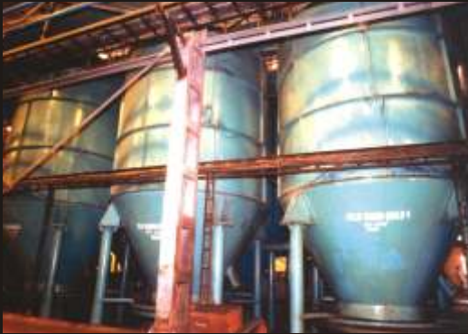
100 Tons/hr Sand Mixing Capacity
