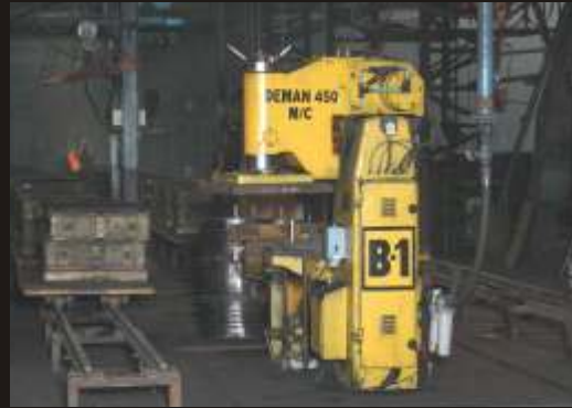
2 sets of ARPA 450 and 1 set of ARPA 900 simultaneous jolt squeeze machine
